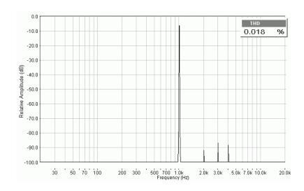
THD @ 100 mW 12 V supply 32 Ohm Load G = 20dB
