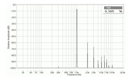
THD @ 750 mW, 12 V supply 8 ohm load G = 20dB
